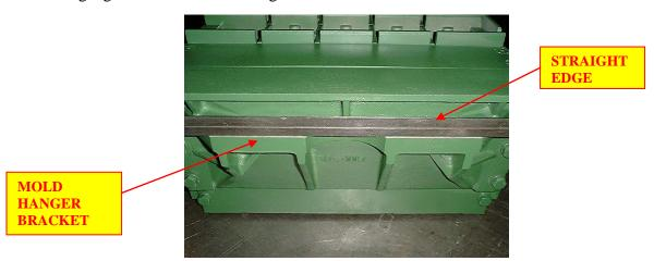
3. To make sure the mold hanger brackets are installed correctly, measure all four corners using a dial caliper, as shown, using the outer holes. Verify measurement of all four corners are the same.
